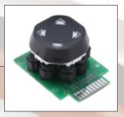
The rocker switch modules RS1 and RS2 are designed to be installed into front panels, multifunction grips or other switching units.
